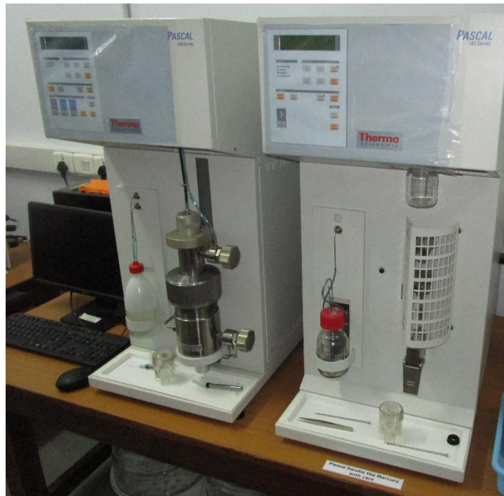
Figure 3.14: MIP setup (Pascal Mercury Porosimeter from ThermoFisher Scientific)
