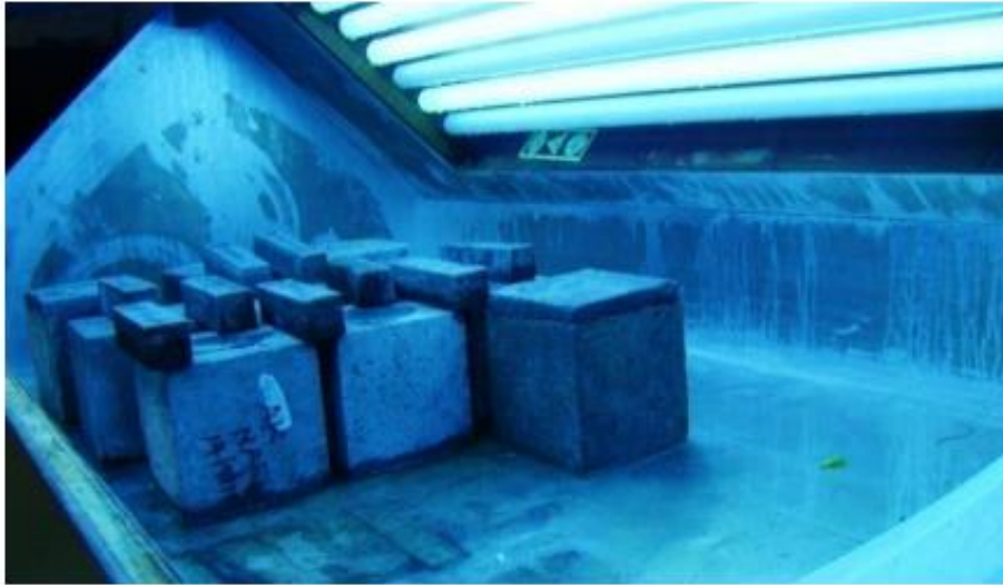
Figure 3.7: Specimens placed in a specially fabricated chamber of 1.5 \times 0.5 \times 0.5 m for accelerated weathering
